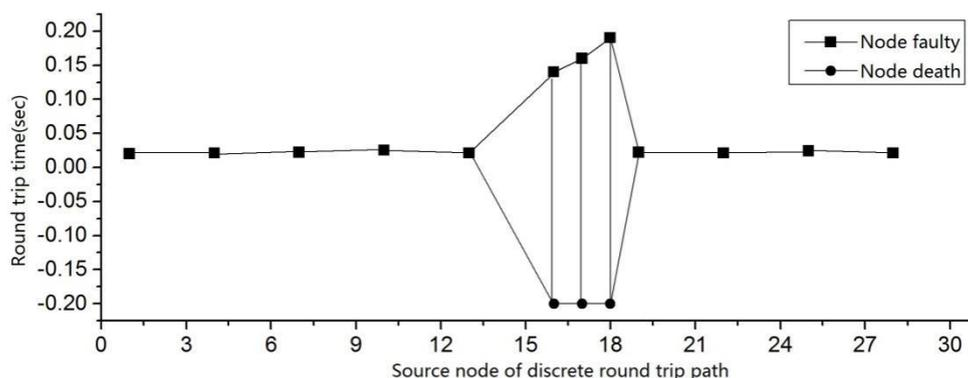
Figure 5. The round trip time chart when 30 nodes and node 18 failed
