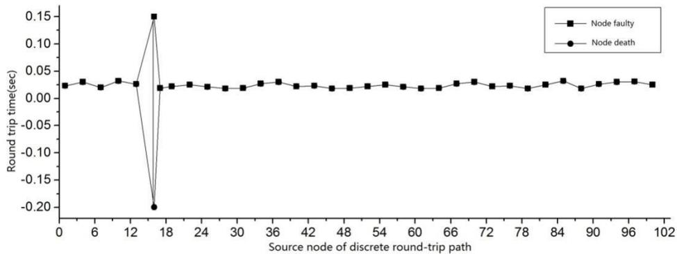
Figure 2. The round trip time chart when 100 nodes and node 16 failed
