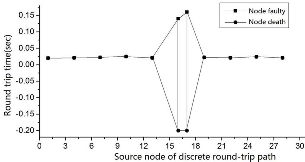
Figure 4. The round trip time chart when 30 nodes and node 17 failed
