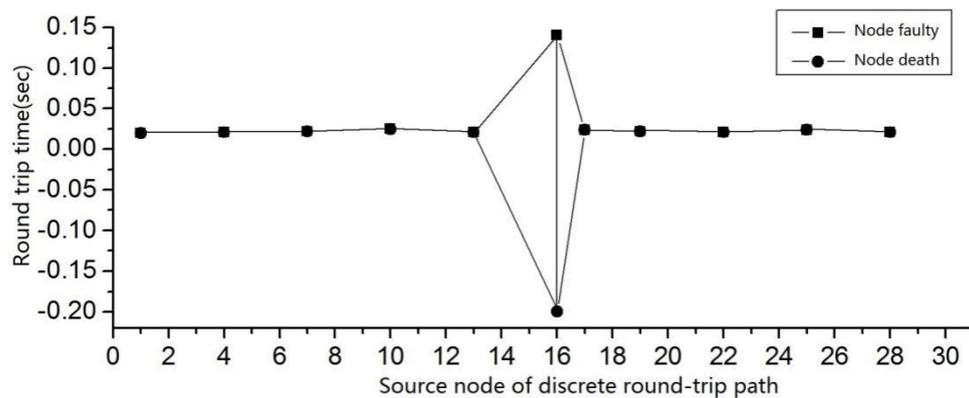
Figure 3. The round trip time chart when 30 nodes and node 16 failed
