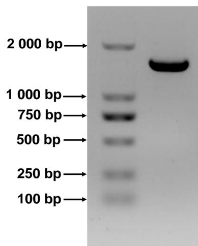
Fig. 1 The electrophoresis for PCR product of MeHXK3 gene M: DNA marker DL2000; 1: PCR product of MeHXK3 gene
