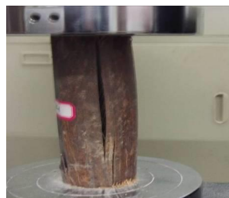
Fig.2 (b) Failure of specimen
