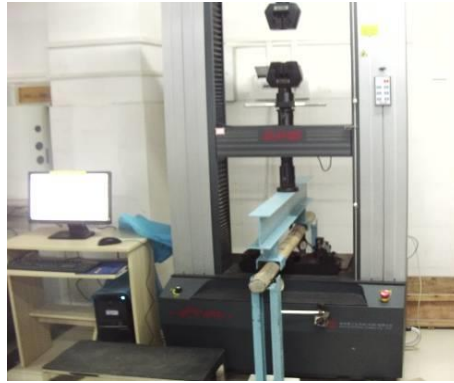
Fig.7 bamboo pipe in bending tests
