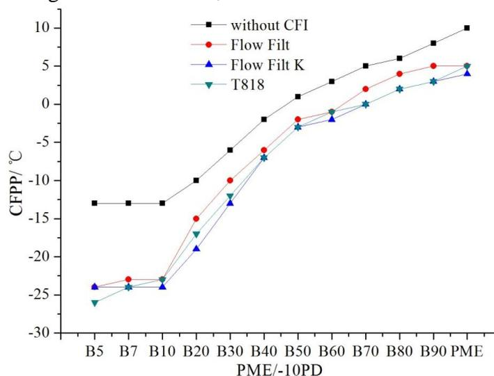
Fig.5 CFPP of PME, PME/-10PD without/with CFI
