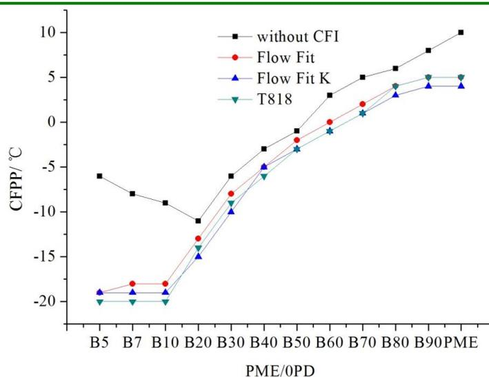
Fig. 4 CFPP of PME, PME/OPD without/with CFI
