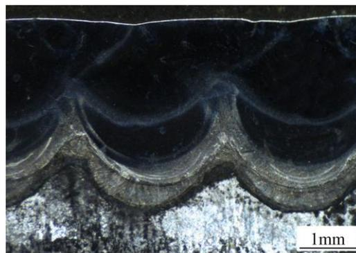
Fig.1 Micromorphology of the gradient wear-resistant coating
