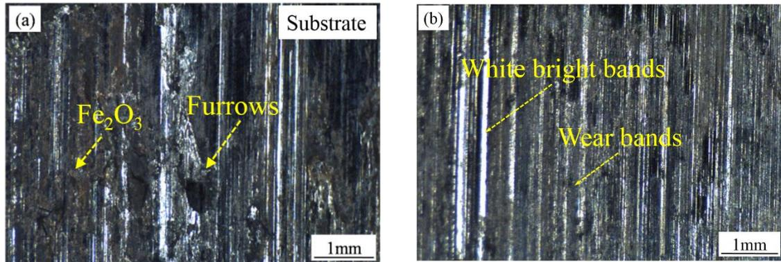
Fig.4 Wear morphologies of the gradient wear-resistant coating
