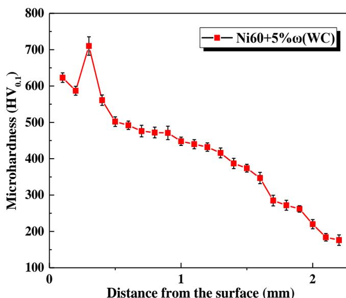
Fig.3 Micro hardness of the gradient wear-resistant coating
