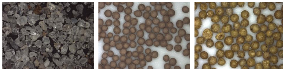
Fig.2 Microscope figures of the three types of prop pants (from left to right: quartz sand, Ceram site, self-suspension proppant)
