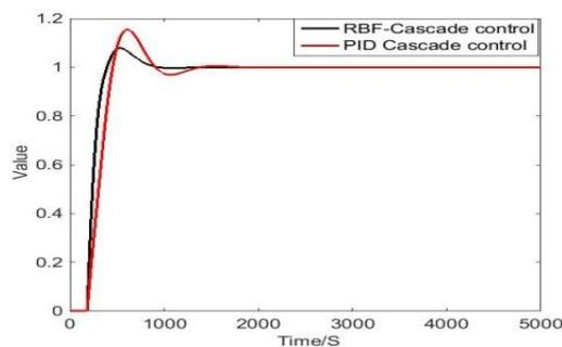
Fig.7 Cascade and cascade - RBF response curve of the time constant mismatch
