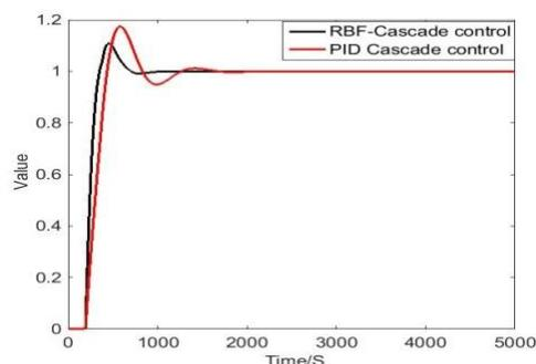
Fig.8 Cascade PID and cascade - RBF response curve of the lag time mismatch
