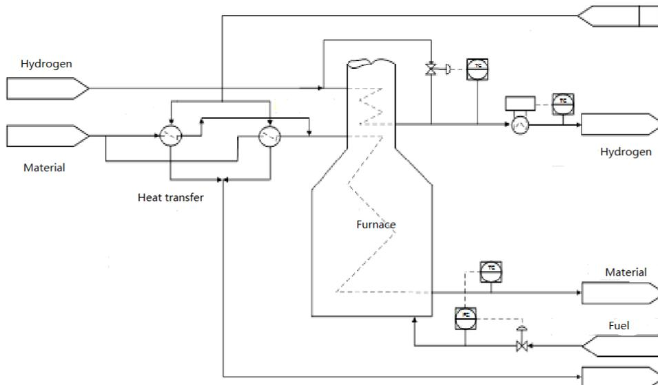
Fig.1 S-Zorb heating furnace temperature control scheme
