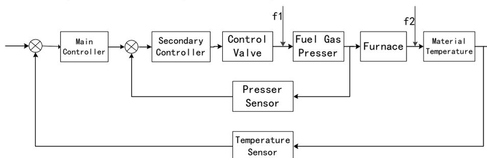
Fig.2 Outlet temperature of the material - the fuel gas pressure cascade control block diagram
