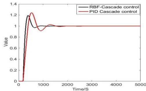
Fig.6 Cascade and cascade - RBF response curve of the ratio coefficient mismatch
