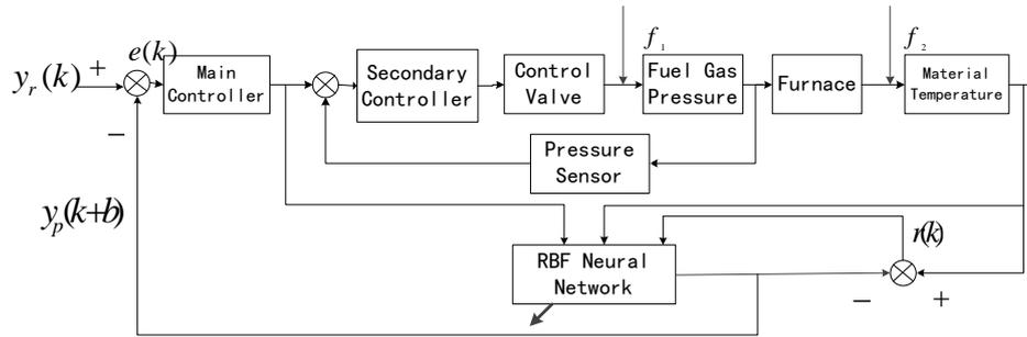
Fig.4 Cascade - RBF neural network predictive control scheme
