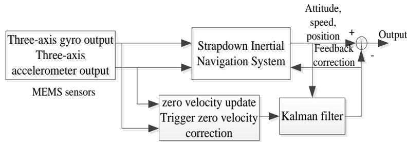
Fig.1 Navigation algorithm structure of PNS
