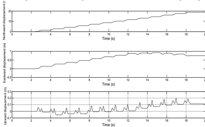
Figure.3 Navigation results of north-walking trajectory
