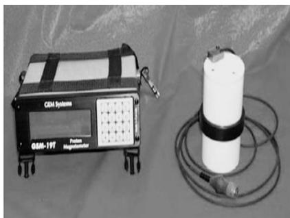
Figure 3 GSM-19T high precision proton magnetometer
