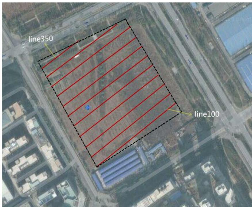
Figure 2 Arrangement plan of the measuring lines
