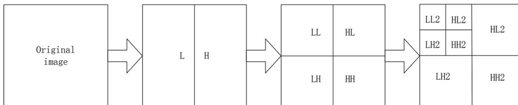
Fig.1 The process of two level image decomposition
