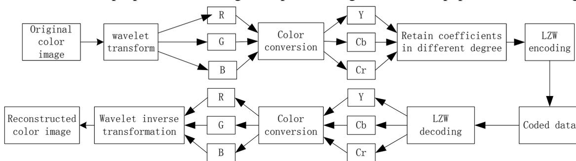
Fig.2: Algorithm Flowchart
