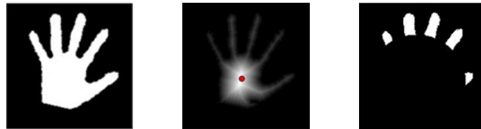
(a) Gesture sub-block (b) Distance shaded image (c) Fingertip part Fig. 10 Fingertip area extraction processing
