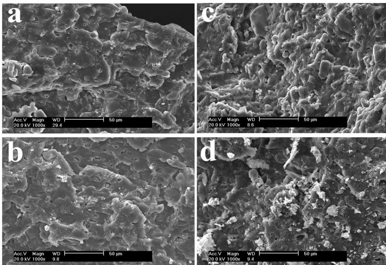
Fig. 3. SEM micrographs of fractured surface of flame-retardant composites a-TPU/IFR; b-TPU/IFR/  $\text{Ni}_2\text{O}_3$ -1.5; c-TPU/IFR/  $\text{Ni}_2\text{O}_3$ -4.5; d-TPU/IFR/  $\text{Ni}_2\text{O}_3$ -7.5.
