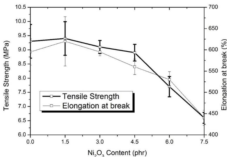
Fig. 4. Mechanical properties of flame-retardant TPU/IFR-Ni<sub>2</sub>O<sub>3</sub> composites
