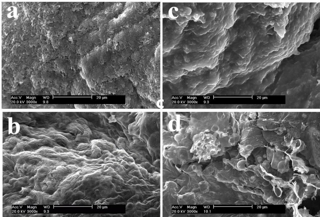
Fig. 2. SEM micrographs of char layers of flame-retardant TPU composites a-TPU/IFR; b- TPU/IFR/ $\text{Ni}_2\text{O}_3$ -1.5; c-TPU/IFR/ $\text{Ni}_2\text{O}_3$ -4.5; d-TPU/IFR/ $\text{Ni}_2\text{O}_3$ -7.5.
