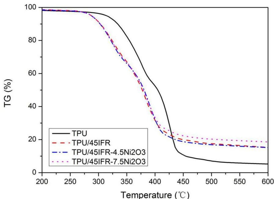
Fig. 1. TG thermograms of flame retardant TPU composites in N<sub>2</sub> atmosphere
