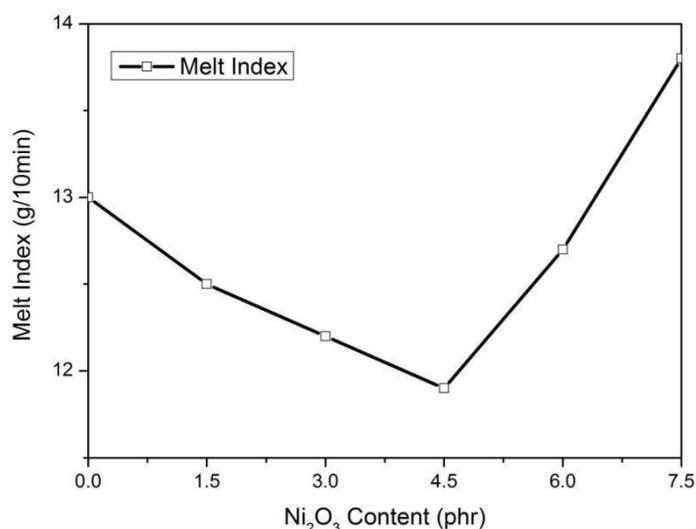
Fig. 5. Variations of MI values of flame-retardant TPU/IFR-Ni<sub>2</sub>O<sub>3</sub> composites at different amounts of Ni<sub>2</sub>O<sub>3</sub>
