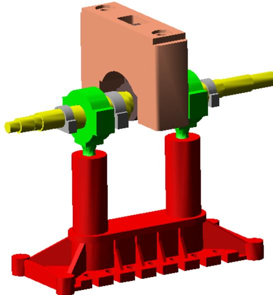
Fig. 2 The three-dimensional model of slider-crank mechanism
