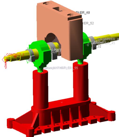
Fig. 3. The model of slider-crank mechanism with boundary conditions and motion
