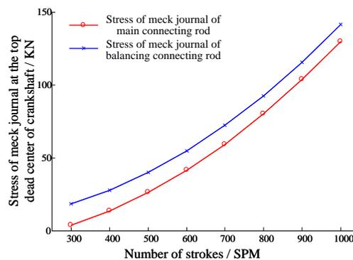
Fig. 7. Stress of the top dead center of crankshaft under different strokes
