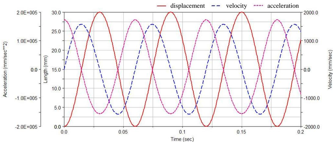
Fig. 4. The displacement, velocity and acceleration in vertical direction of slider under 1000 SPM
