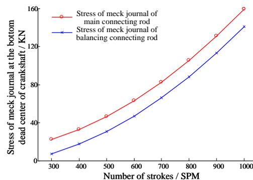
Fig. 8. Stress of the bottom dead center of crankshaft under different strokes
