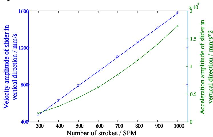
Fig. 5. The curve of velocity and acceleration amplitudes of slider under different strokes
