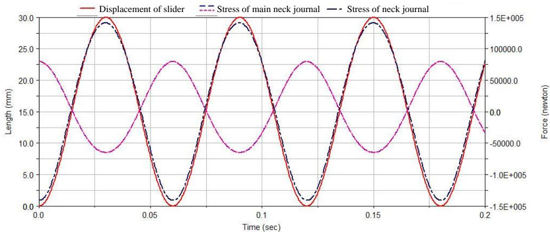
Fig. 6. The stress in vertical direction of crankshaft under 1000 SPM
