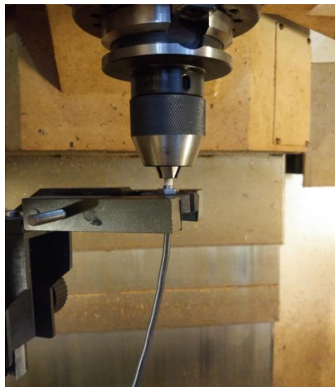
Fig.7 Installation of DT3005 displacement sensor
