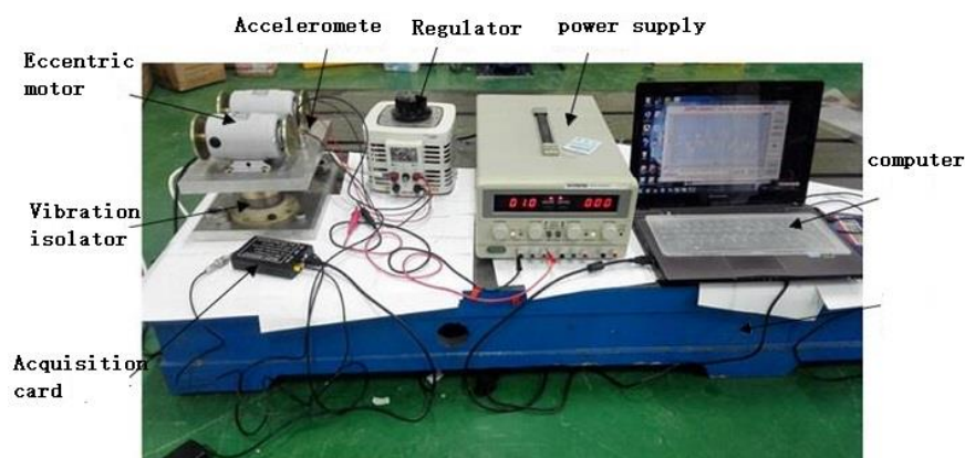
Fig. 3 Vibration isolation test platform
