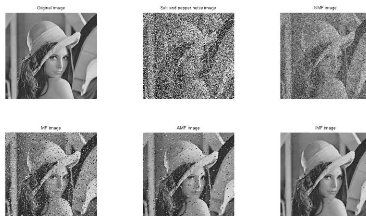
Fig.2 Processing results of 50% salt and pepper noise images with different algorithms.
