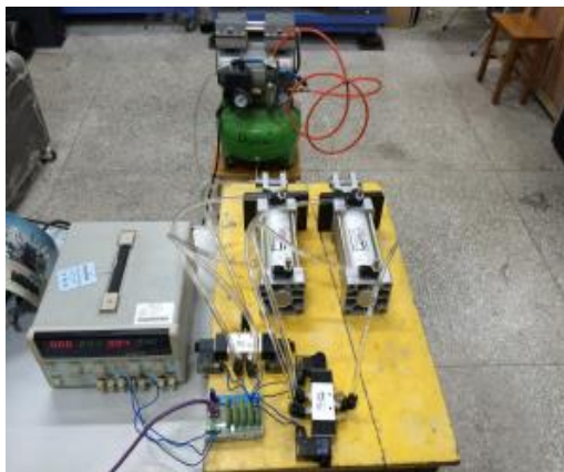
Figure 5 Cylinder control physical hardware wiring
