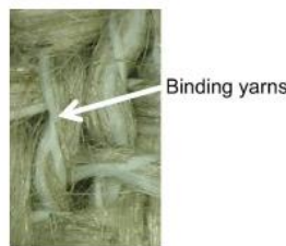
Fig. 13. Unidirectional flax roving with binding polyester yarn in the low twist twill textile. (For interpretation of the references to colour in this figure legend, the reader is referred to the web version of this article.)
