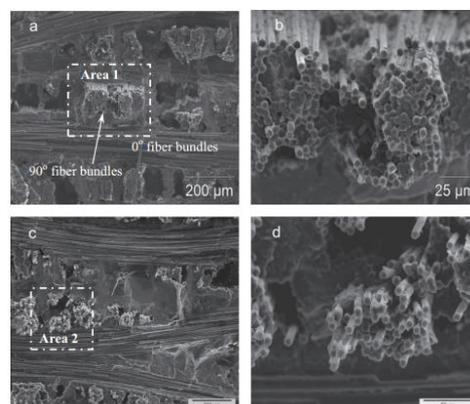
Fig. 7. The fracture surface of C/C–SiC composites (SEM images, topography contrast), (a) The virgin sample; (b) The magnification of Area 1; (c) The fatigued sample after 105 cycles with 83% stress level; (d) The magnification of Area 2.
