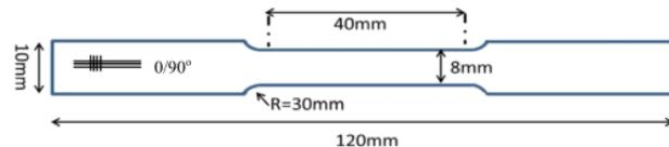
Fig. 1. Geometry of the tension specimens.
