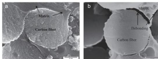
Fig. 8. SEM image of the interface between carbon fiber and matrix in virgin and pre-fatigued sample, (a) Intact interface in the virgin sample; (b) Interfacial debonding in the pre-fatigued sample.
