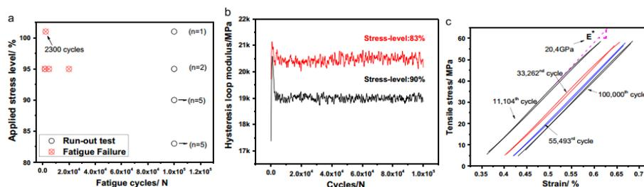
Fig. 2. (a) Tensile fatigue life S–N curve of the C/C–SiC composites; (b) Hysteresis modulus versus cycles; (c); Stress–strain hysteresis loop with stress level of 83%. The horizontal arrows indicate the samples that achieved all 105 cycles, n in the bracket indicates the number of valid samples and  $E^*$  is the hysteresis loop modulus.
