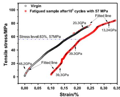
Fig. 4. Typical tensile stress–strain curves of C/C–SiC composites before and after 105 cyclic loading with stress level of 83%.
