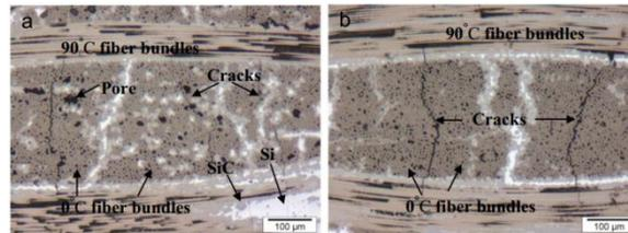
Fig. 3. Typical optical microstructures of C/C–SiC before/after fatigue, (a) Sample before fatigue; (b) Sample after fatigue with stress level 83% after 105 cycles.
