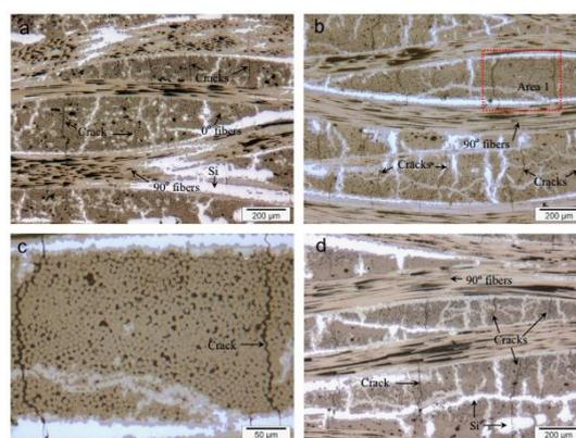
Fig. 5. Crack density and distribution in the C/C–SiC composites, (a) Microstructure before fatigue; (b) microstructure after fatigue with a stress level of 83%; (c) microstructure after fatigue with a stress level of 90%.
