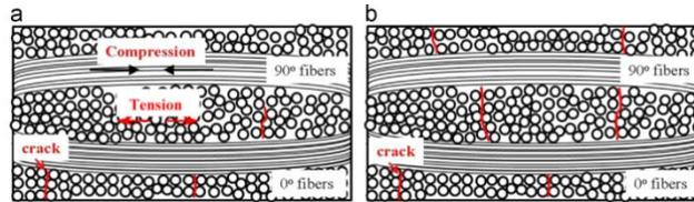
Fig. 6. Schematic sketch of the cracks caused by thermal residual stresses in C/C–SiC composites before/after fatigue, (a) C/C–SiC composites without fatigue load; (b) C/C–SiC composites after fatigue load. The black arrows in Fig. 6(a) indicate the compressive stresses, and the red arrows indicate the tensile stresses.
