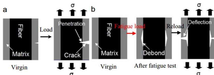
Fig. 9. Crack propagation schematic in basic cell of the C/C–SiC composites, (a) Crack penetration in a virgin sample; (b) Crack deflection in a pre-fatigued sample.
