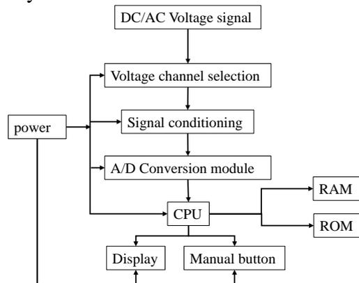
Fig.4 the hardware block diagram of the high frequency data acquisition system for buried steel pipelines
