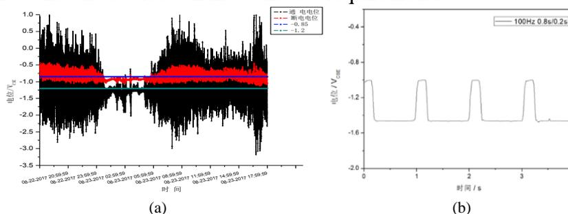
Fig.8 The (a) fluctuation of buried pipelines under subway influence (b) buried pipeline with potential
