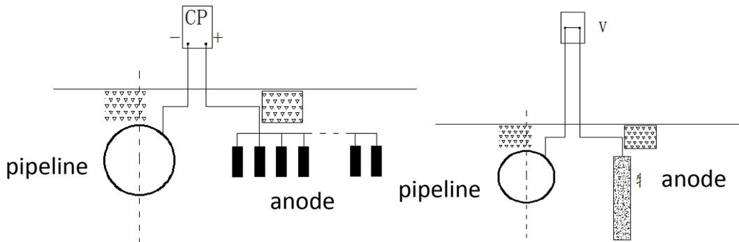
Fig.2 Schematic diagram of the principle of forced current cathodic protection
