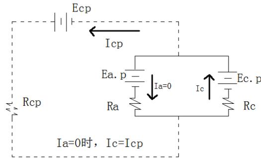
Fig.1 Basic principle diagram of cathodic protection
