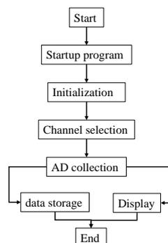
Fig. 5 general design block diagram of system software
