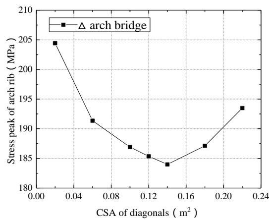
Fig. 16 Combined stress change curve of arch rib with variable CSA of diagonal under combined load
