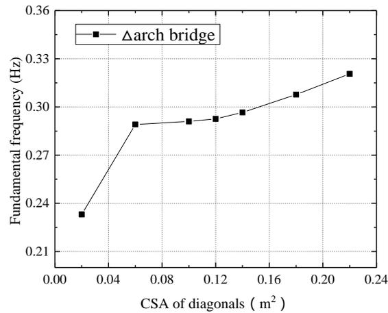
Fig. 18 Fundamental frequency change curve with variable CSA of diagonal
