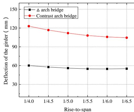
Fig. 26 Deflection change curve with variable rise-to-span ratio
