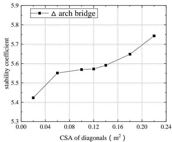
Fig. 17 Stability change curve with variable CSA of diagonal
