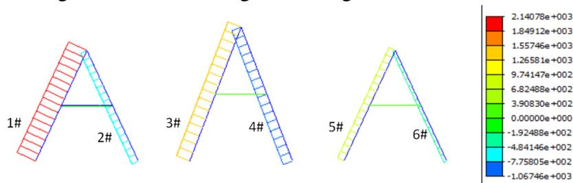
Fig. 11 Axial force diagram of diagonal under live load
