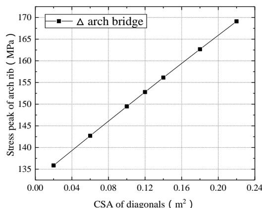
Fig.14 Stress change curve of arch rib with variable CSA of diagonal under dead load
