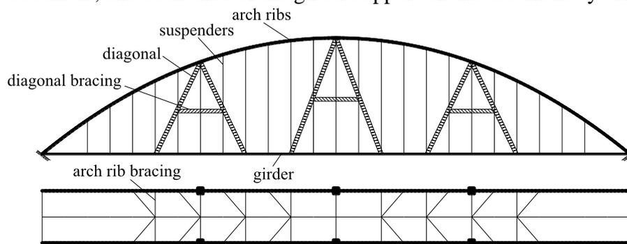
Fig. 1 Structural style of  $\Delta$  arch bridge
