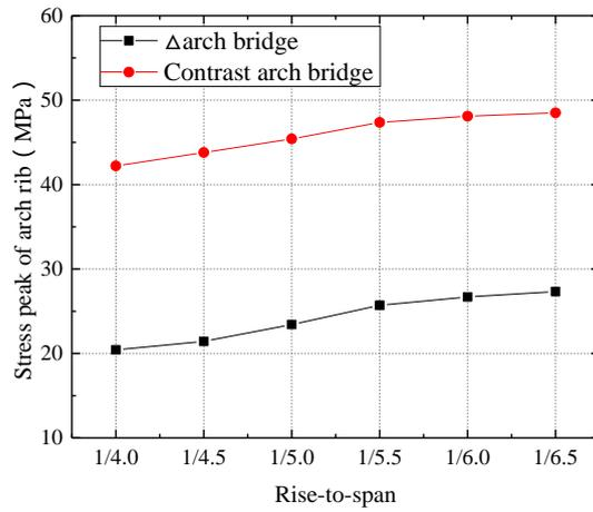
Fig. 22 Stress change curve of arch rib with variable rise-to-span ratio under live load
