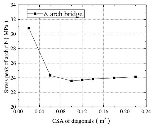
Fig.15 Stress change curve of arch rib with variable CSA of diagonal under live load
