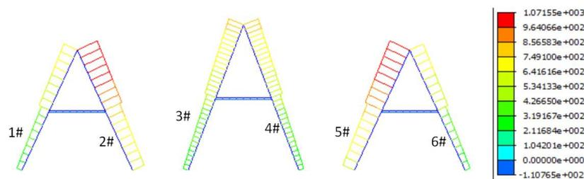
Fig. 10 Axial force diagram of diagonal under dead load
