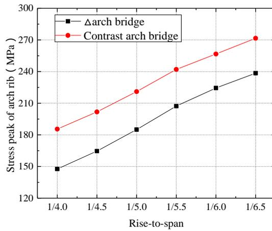
Fig. 23 Stress change curve of arch rib with variable rise-to-span ratio under combined load
