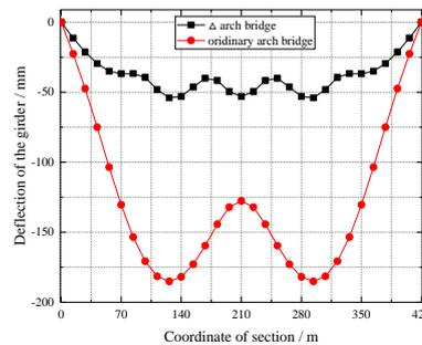
Fig. 9 The displacement envelope diagram of the girder of  $\Delta$  arch bridge and ordinary bridge under live load
