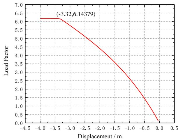
Fig. 12 Load-displacement curve of contrast arch bridge
