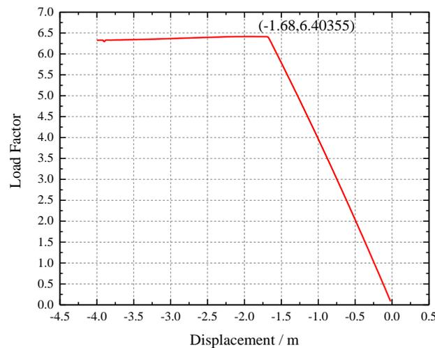
Fig. 13 Load-displacement curve of  $\Delta$  arch bridge
