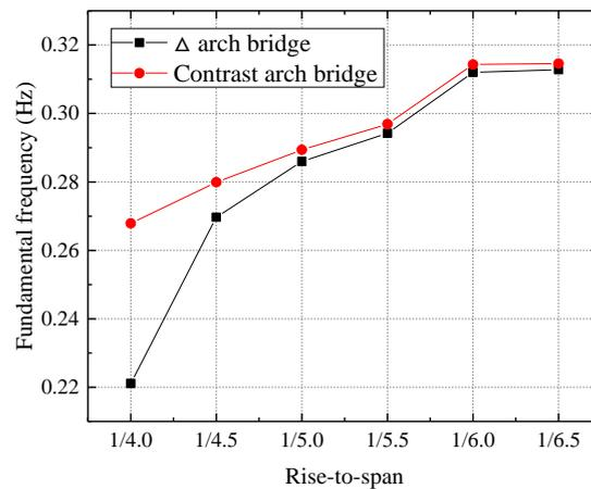
Fig. 25 Fundamental frequency change curve with variable rise-span ratio
