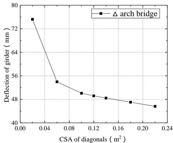
Figure 19 Deflection change curve with variable CSA of diagonal
