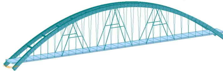
Fig. 6 Model of  $\Delta$  Arch Bridge
