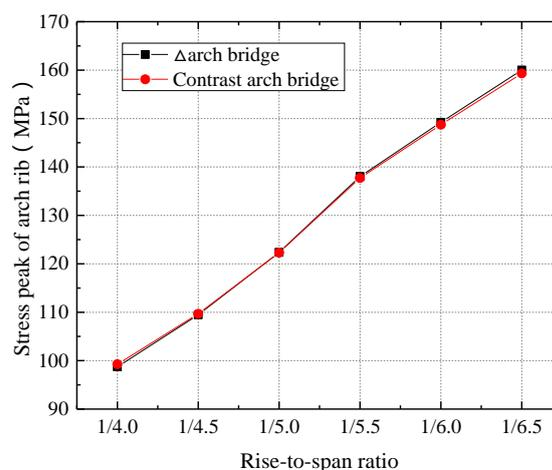
Fig. 21 Stress change curve of arch rib with variable rise-to-span ratio under dead load
