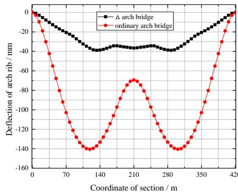
Fig. 8 The displacement envelope diagram of arch rib of  $\Delta$  arch bridge and ordinary bridge under live load
