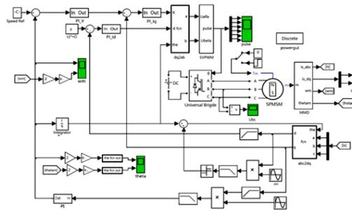
Fig.3 System simulation structure diagram
