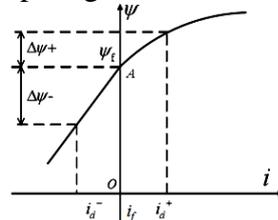
Fig.2 Direct axis magnetic circuit  $\psi$ - $i$  characteristic curve
