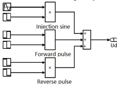
Fig.4 Voltage signal injection module
