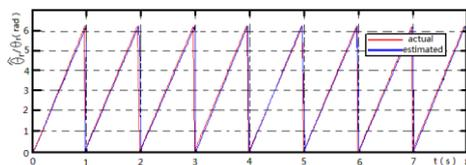
Fig.8 (a) Rotor position
