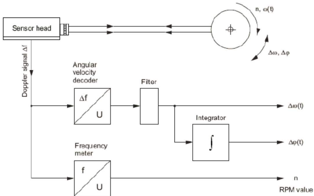
Fig. 3 The working principle of laser torsional vibration measurement system
