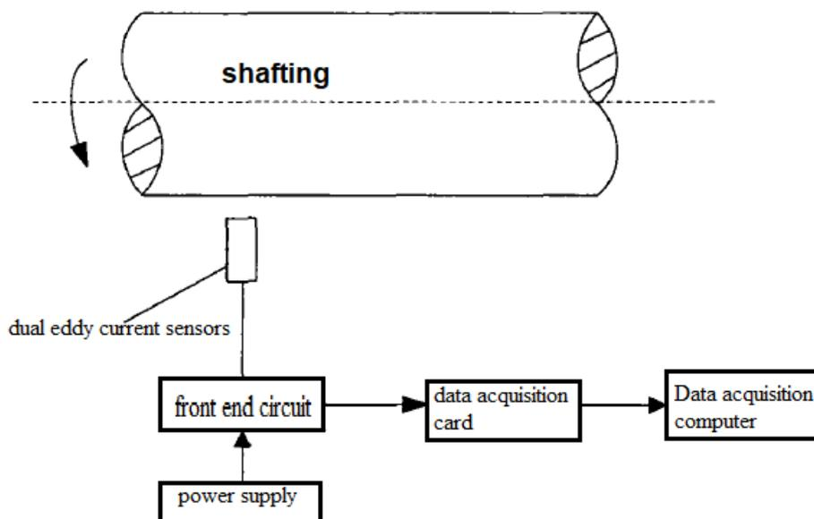
Fig.4 The signal acquisition device for whirling vibration of shafting
