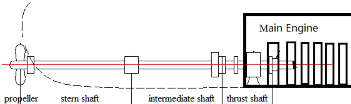
Fig. 1 The schematic diagram of the propulsion shafting
