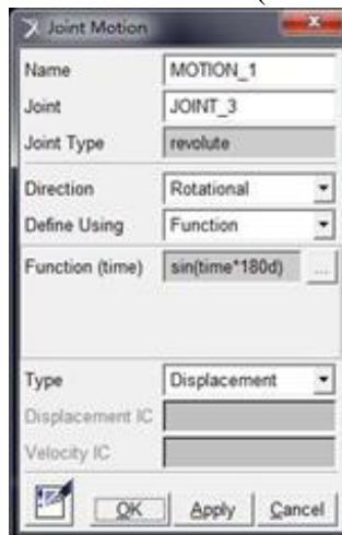
Fig. 3 Simulation setting of turntable pitching motion
