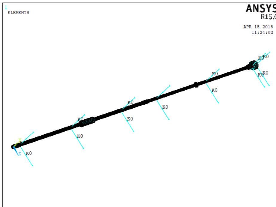
Fig.1. Finite element model of the propulsion shafting
