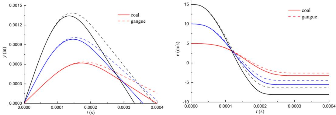
Fig.3 Normal displacement - time history of rock Fig.4 Normal velocity - time history rock
