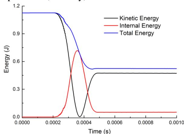
Fig.2 Energy-time history of coal at impact velocity 5m/s
