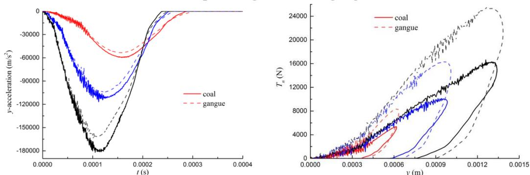
Fig.5 Normal acceleration-time history of rock Fig.6 Contact force-displacement curve of rock
