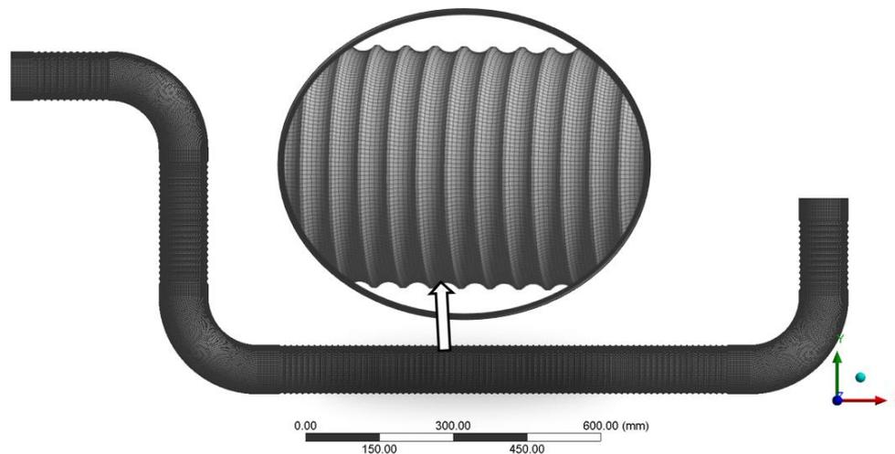
Fig. 6 Grid of the fluid calculation domain
