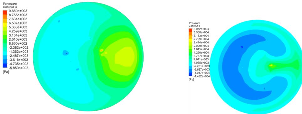
(a) smooth pipeline (b) the non-smooth inner wall of the convex hull
