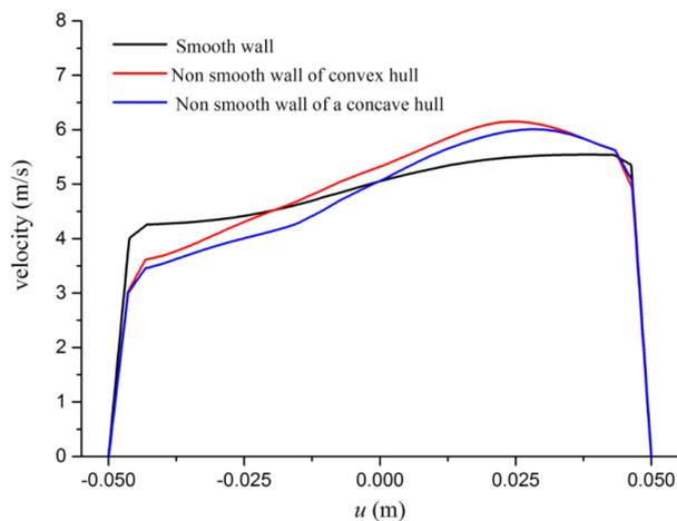
Fig.10. Fluid velocity at the outlet of the pipe
