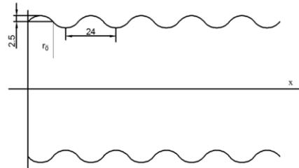
Fig. 2. Non-smooth surface of earthworm
