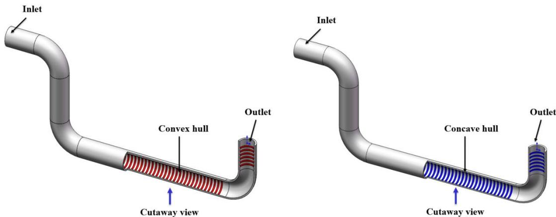
(a) Non-smooth wall pipe with convex hull (b) Non-smooth wall pipe with concave hull
