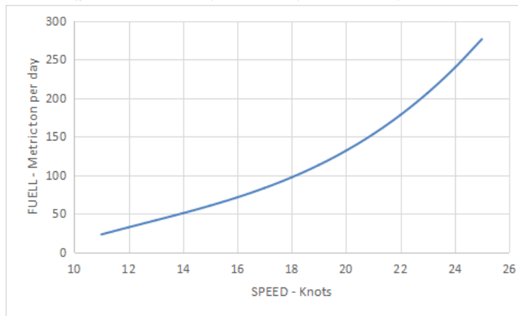
Figure 2 The baseline of the ships between the speed and the fuel consumption
