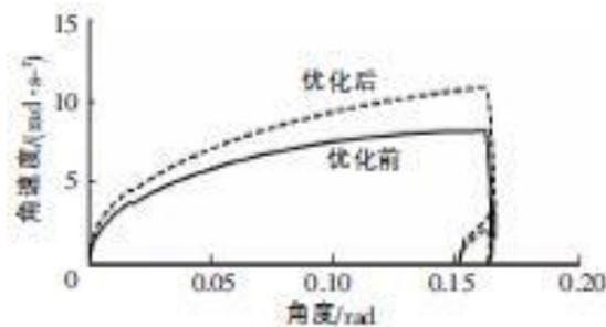
Fig.10 Before and After Optimization of Spindle Angular Velocity Changes
