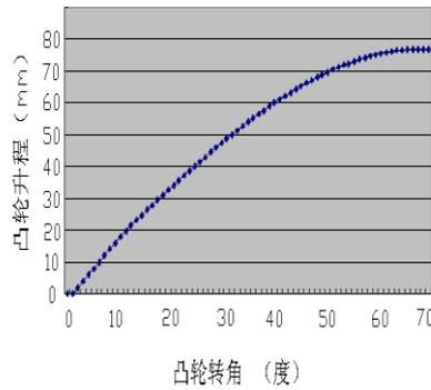
Fig. 3 Cam Rise Curve
