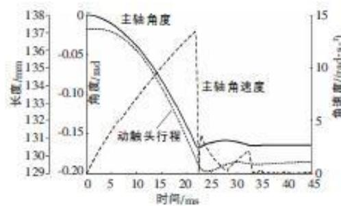
Fig. 8 Opening Characteristics before Optimization
