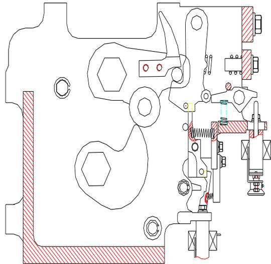
Fig. 1 Spring Operating Mechanism Structure Program
