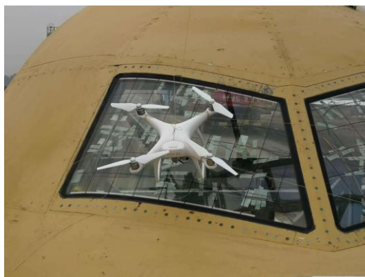
Fig.4 The first collision Test between UAV and Civil Aviation passenger aircraft [9]
