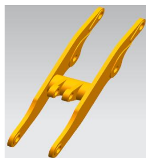
Fig 7. The three-dimensional model of swing arm
