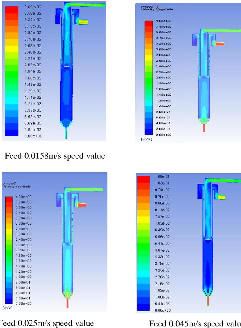
Fig. 4 distribution of flow field at different feed speeds
