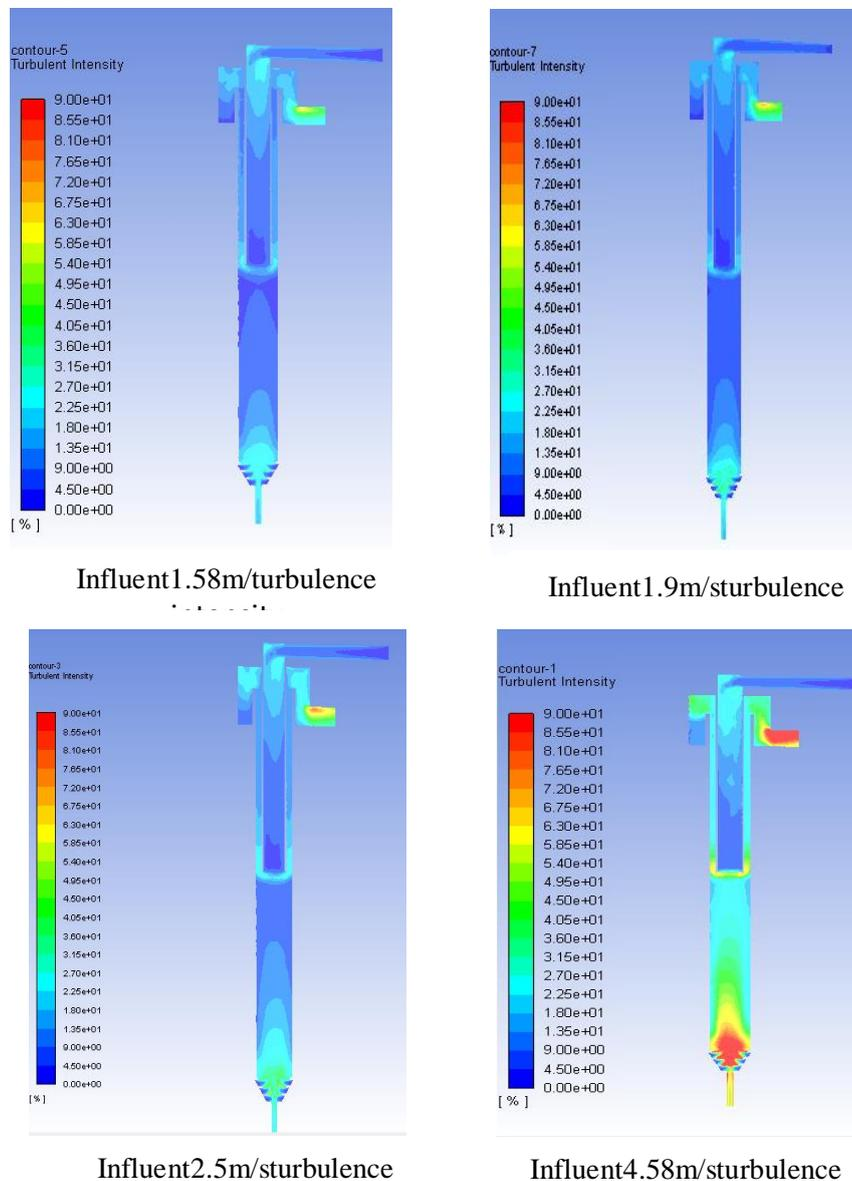
Fig. 3 turbulence intensity x-z plan
