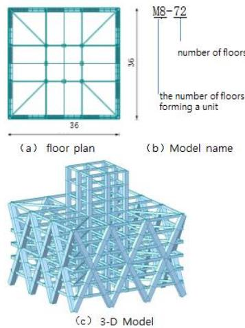
Figure 1. Basic Structural Model
