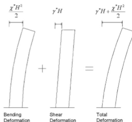
Diagram 1: Shearing and Bending Deformation of High-rise Building
