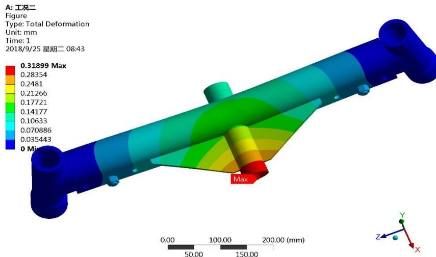
Fig. 3 Front axis overall deformation cloud
