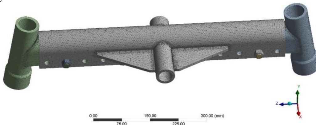
Figure 1 front-axis model meshing results
