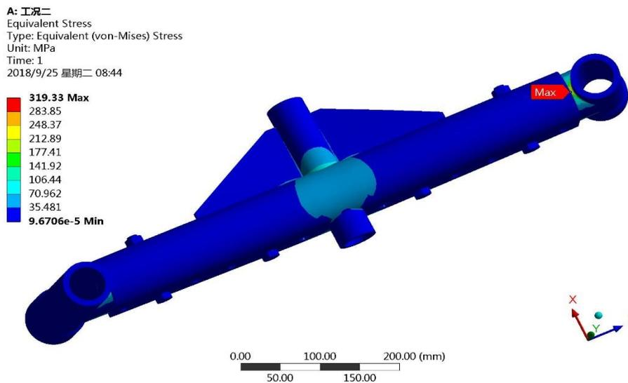
Fig.2 Front axle overall force cloud map
