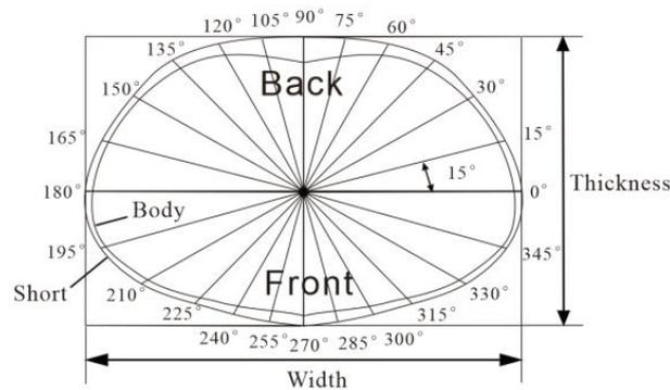
Fig.1 Selection of morphological index of characteristic cross-section
