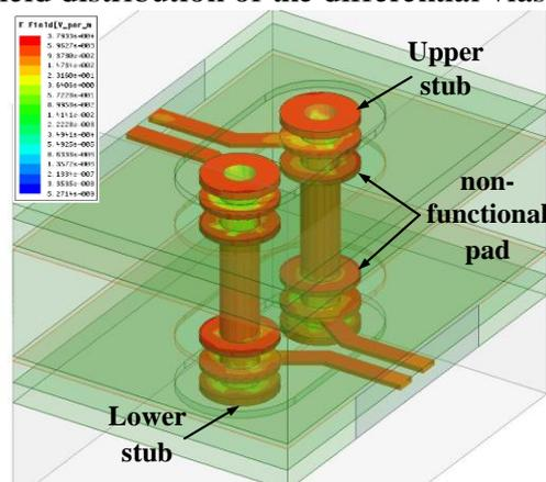
Fig.3 Differential vias electric field distribution
