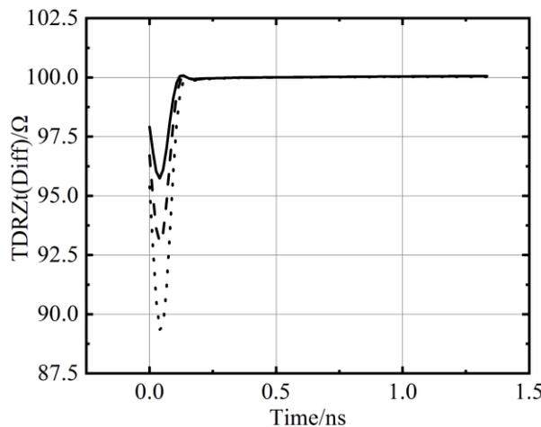
Fig.5 Differential impedance change comparison
