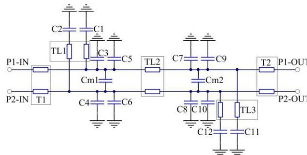
Fig.2 Differential vias circuit model
