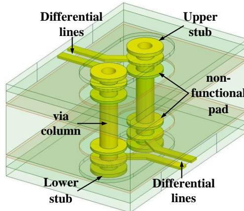
Fig.1 Differential vias physical model
