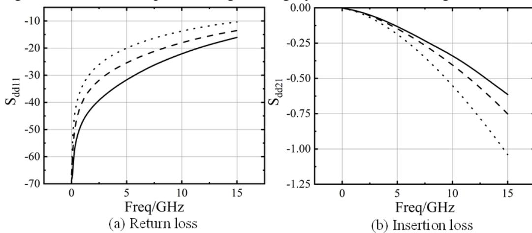
Fig.4 Return loss and the insertion loss of the differential vias.
