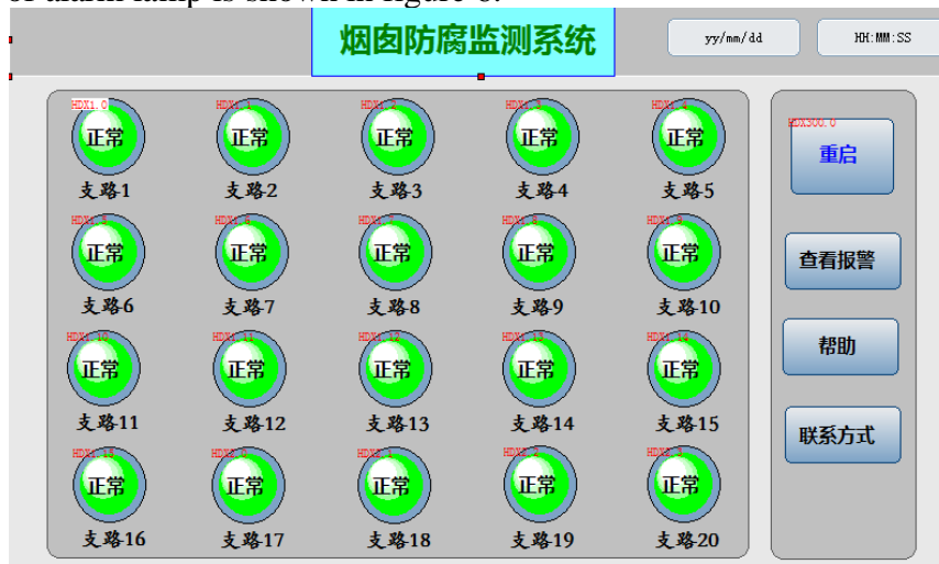
Fig. 6 Display interface of alarm lamp
