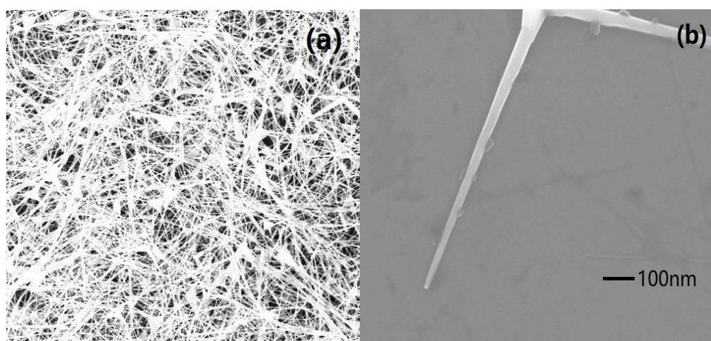
Fig. 1. (a) SEM image of ZnO nanomaterial (b) SEM image of graphene QDs/ZnO nanostructure.
