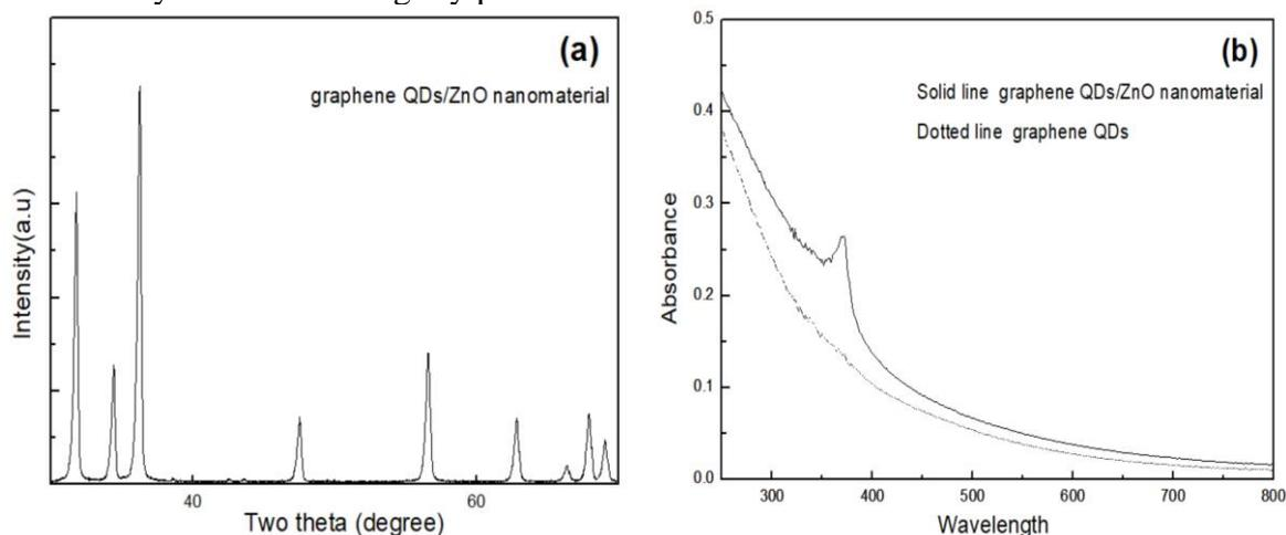
Fig. 2. (a) XRD patterns of graphene QDs/ZnO nanomaterial. (b) UV-vis spectra of graphene QDs/ZnO nanomaterial
