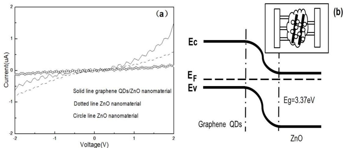
Fig. 3. (a) I-V characteristics of the fabricated samples measured at room temperature (b) Mechanism for graphene QDs compounded with ZnO nanomaterial. Higher inset: top view of the fabricated sample.
