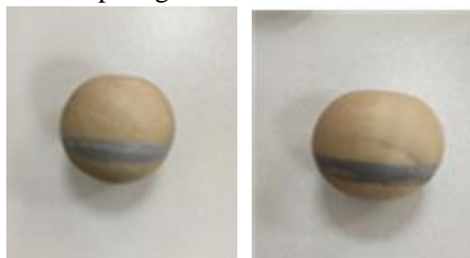
Fig. 9 Frac ball in seat (after compression)
