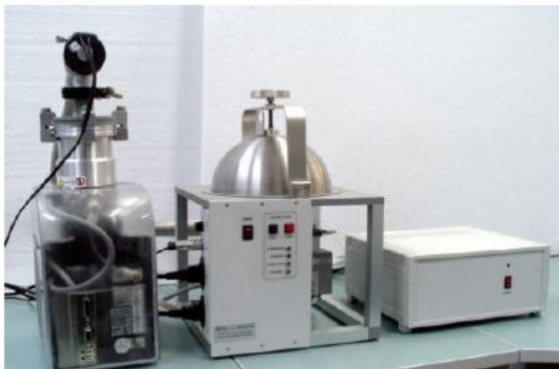
Fig. 3 test system of Russian z-meter semiconductor refrigeration sheet
