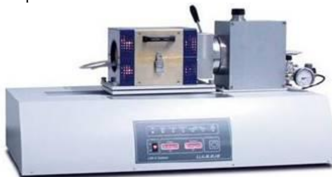
Fig. 2 test system of Lindsey semiconductor refrigeration sheet
