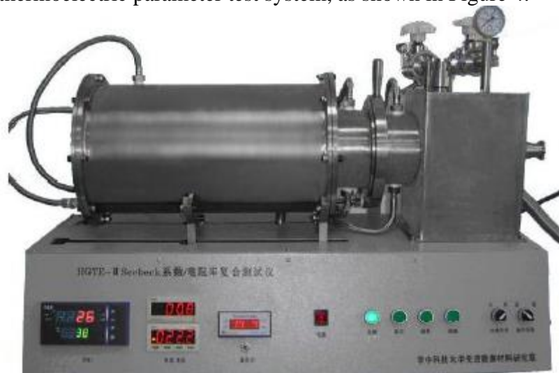
Fig. 4 hgte-ii thermoelectric parameter test system
