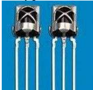
Figure3 physical figure of infrared remote control receiver module
