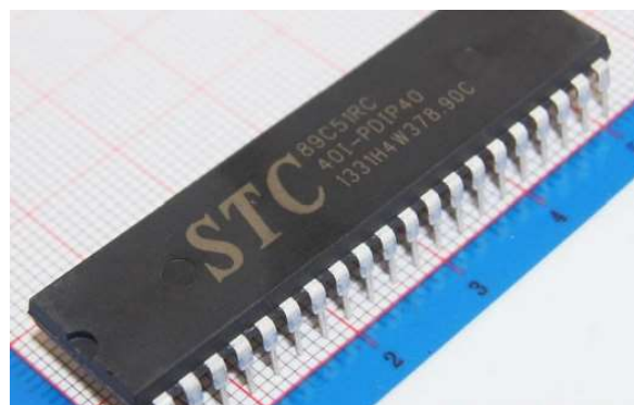
Figure1 physical figure of STC89C51 single chip microcomputer
