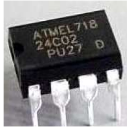
Figure 2 physical figure of AT24C02 memory chip module
