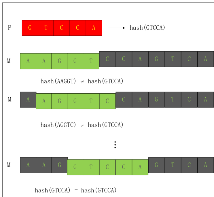
Fig 2. The example of KR algorithm. P is pattern string and M is the main string.
