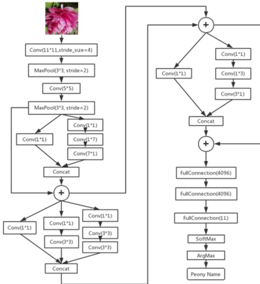
Figure 2. The overall structure of Inception-Alexnet
