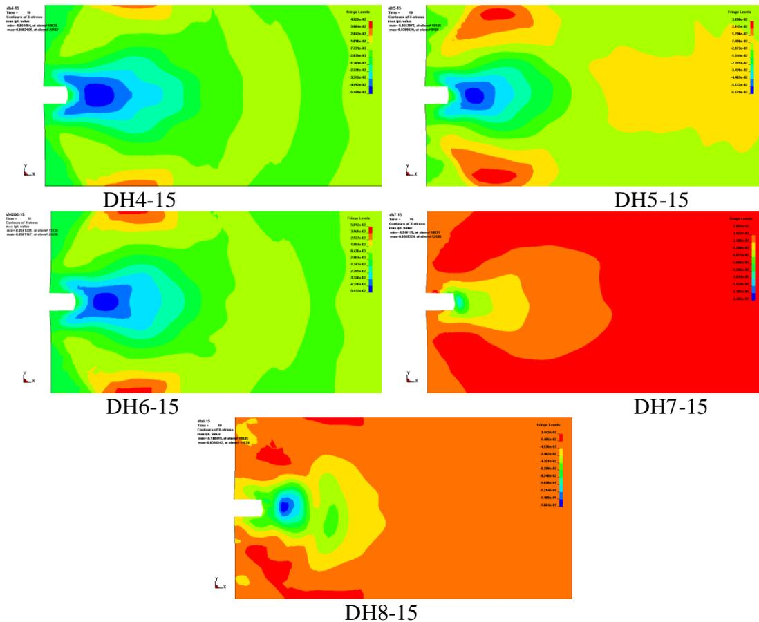
Fig.2 Stress model of rock mass under different jet diameters at the same well depth at 10ms
