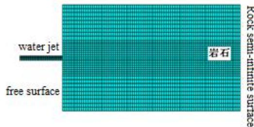
Fig. 1 Impacting rock model by pressure water jet
