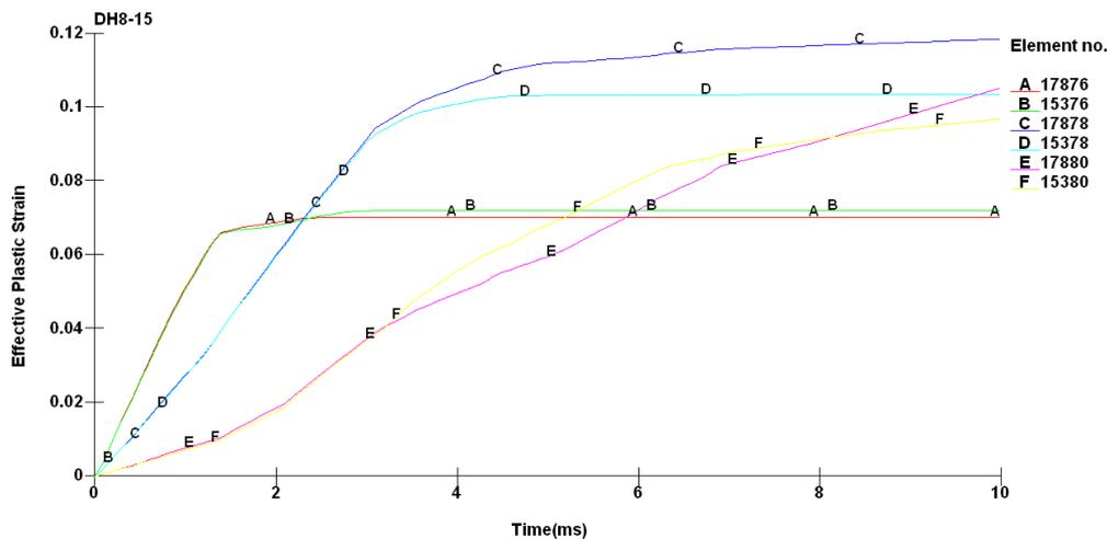
Fig.4 Plastic strain time history curve of jet diameter 8mm
