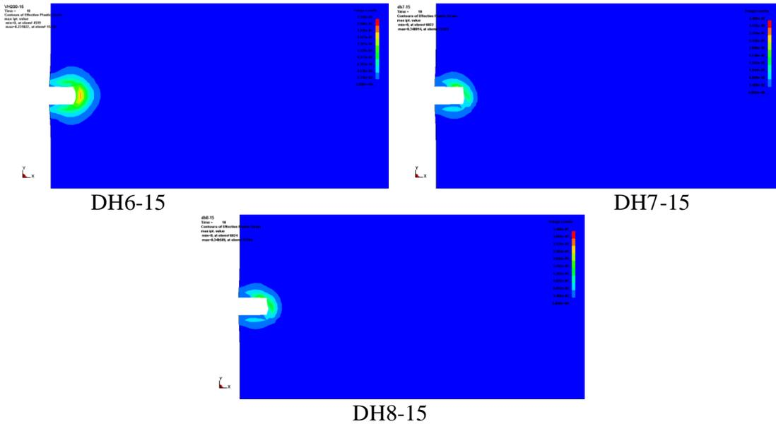
Fig.3 Equivalent plastic strain cloud diagram of rock mass under different jet diameters at the same well depth at 10ms
