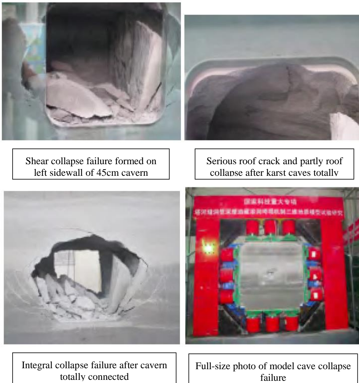
Fig. 6 Model cave collapse failure process
