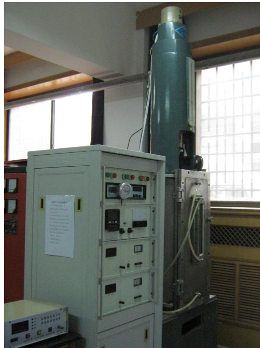
Fig. 1 Schematic diagram of the experiment equipment for crystal growth. The experiment equipment is composed of vacuum device (a rotary and a diffusion pump) and growth chamber.
