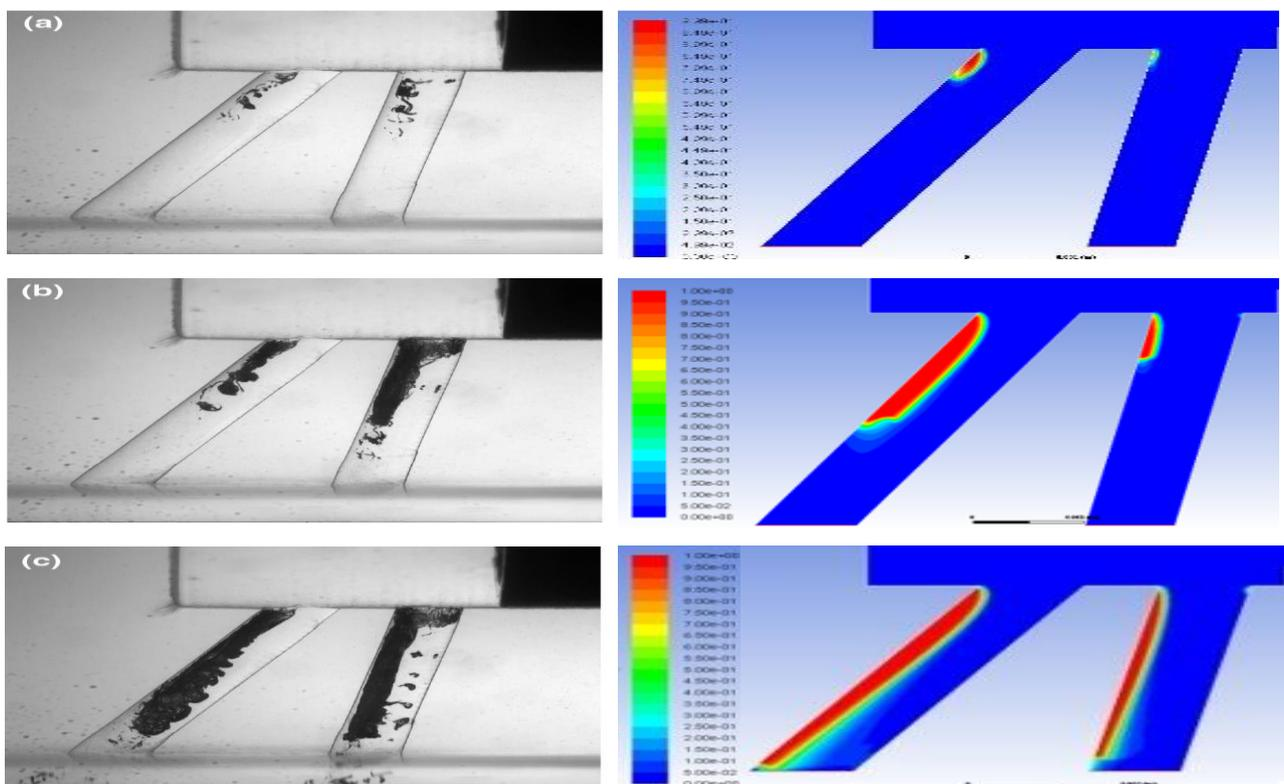
Fig. 9 Comparison of internal flow simulation and experimental results of dual-hole nozzle
