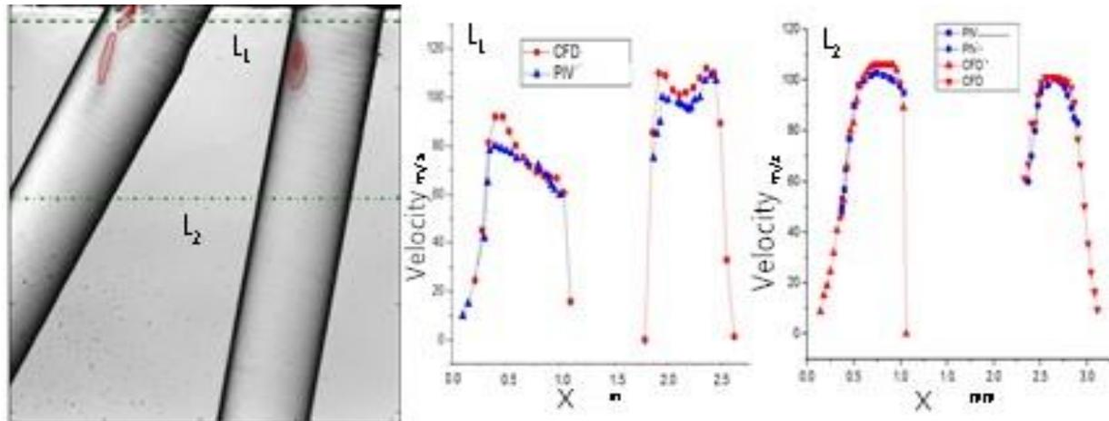
Fig. 10 Comparison of PIV Measurement and Simulation with the Cavitation Number of 1.3
