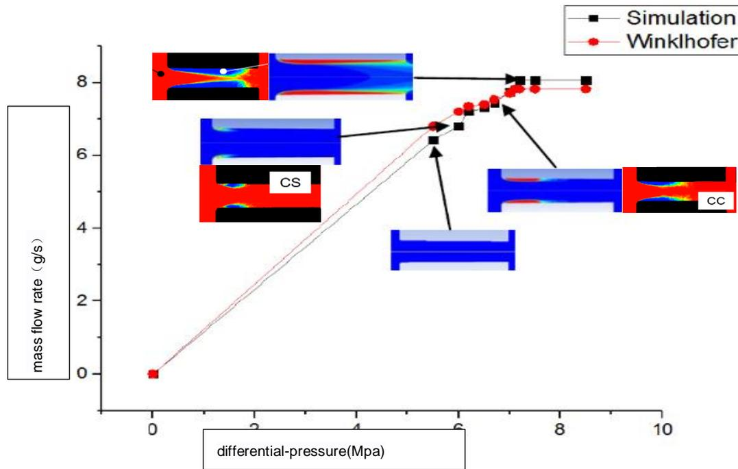
Fig. 3 Comparison of flow rate between simulation and experiment
