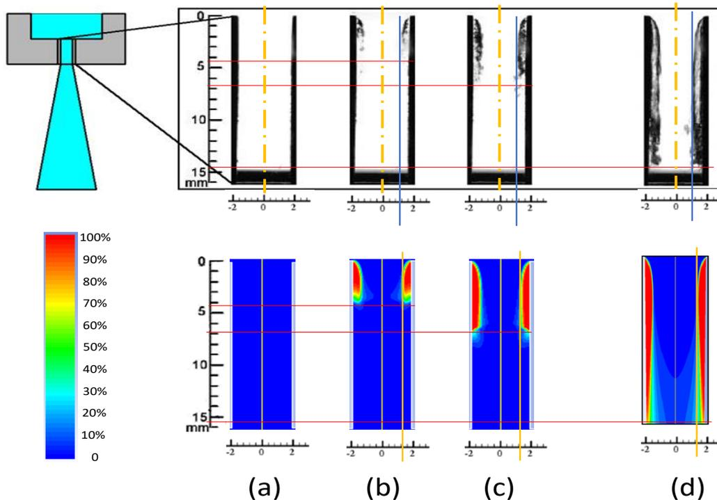
Fig. 6 Cavitation structure in the hole of experiments and simulation
