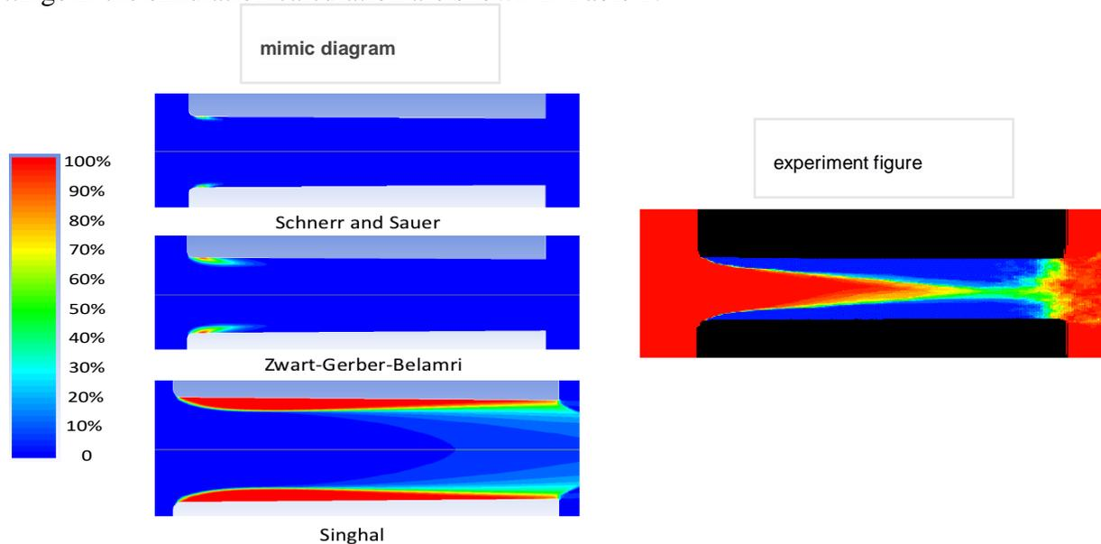
Fig. 2 Comparison of calculation results of different hole models
