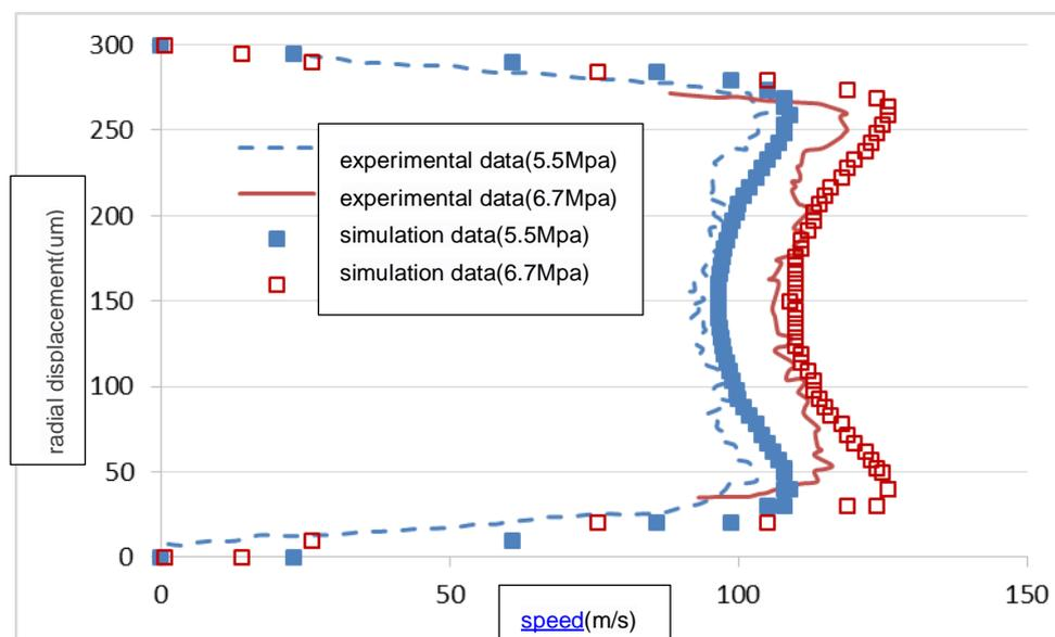
Fig. 4 Comparison of simulation and experimental results of nozzle internal velocity
