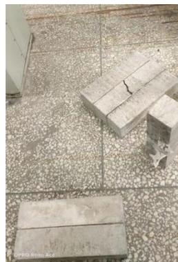
Fig.7 Concrete Flexural Strength Test Fig.8 Flexural Test Specimens
