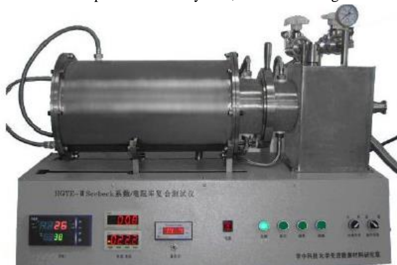
Fig. 4 hgte-ii thermoelectric parameter test system
