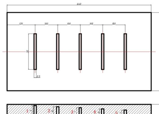
Fig.4 Specimen with artificial defects
