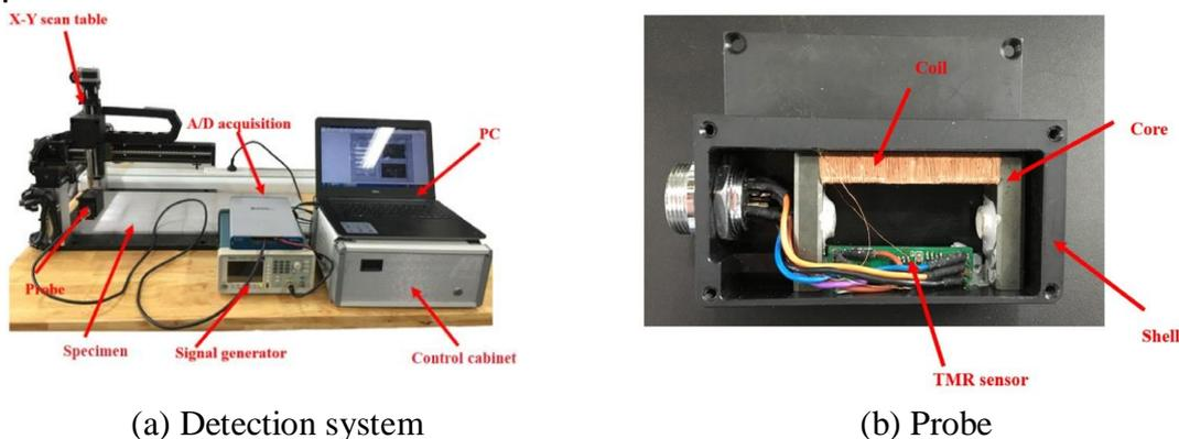
Fig.3 The Detection system and probe
